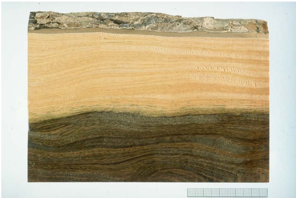
Figure1. Longitudinal section of wood with bark, sapwood and heartwood, Guaiaci lignum; species: Guaiacum sanctum , (copyright BfN).
