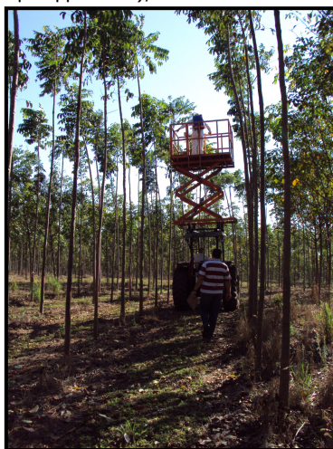
Pantograph type platform used for mahogany drill management experiment in São José do Rio Preto (SP), Brazil. Photo by: Orlando Ohashi
