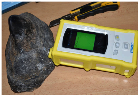
Measuring of the false rhinoceros horn using a Raman spectrometer (photo: Dominika Formanová)
